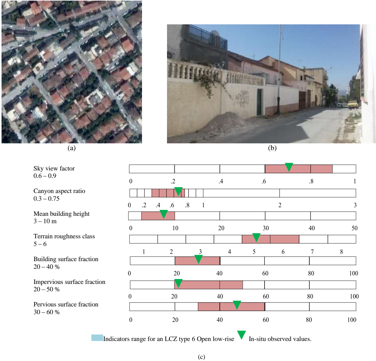
Fig-8. (a). Airborne view of LCZ 6 (b) Street view in LCZ 6 (c) Indicators values for the LCZ 6
