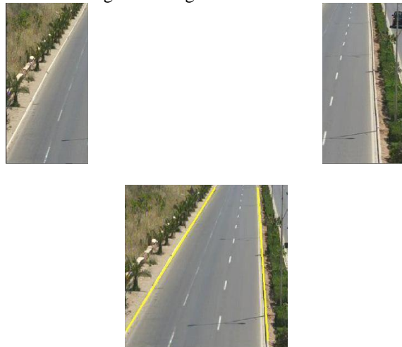
Figure. 3. Road modeling using Hough Transform
