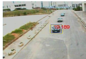
Figure. 9. Mean speed estimation results.
