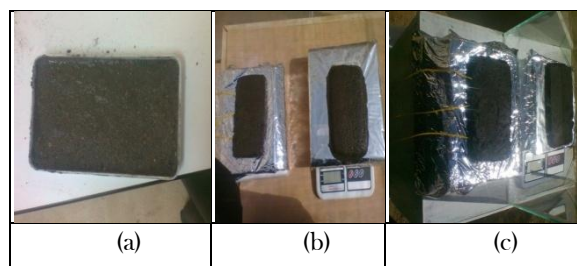
Figure 1. Sample preparation: (a) the phosphate in the block, (b) the phosphate sample under greenhouse, (c) the phosphate sample in open sun
