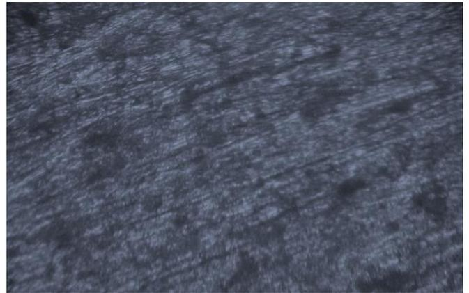
Figure 3: AL 6063 + 7% Si-C, (200+ magnification)
