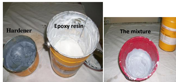
Fig 2. Components of the epoxy resin used.
