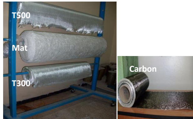
Fig 1. Different types of reinforcements used.
