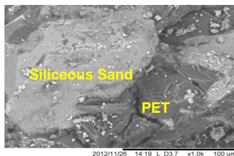
Fig 6. Microstructure of the PET- siliceous sand interface in the samples of the WPLA composite using SEM.
