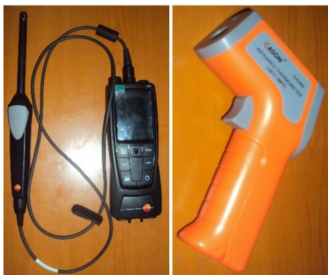
Fig. 6 : Measuring instrument TESTO and infrared thermometer
