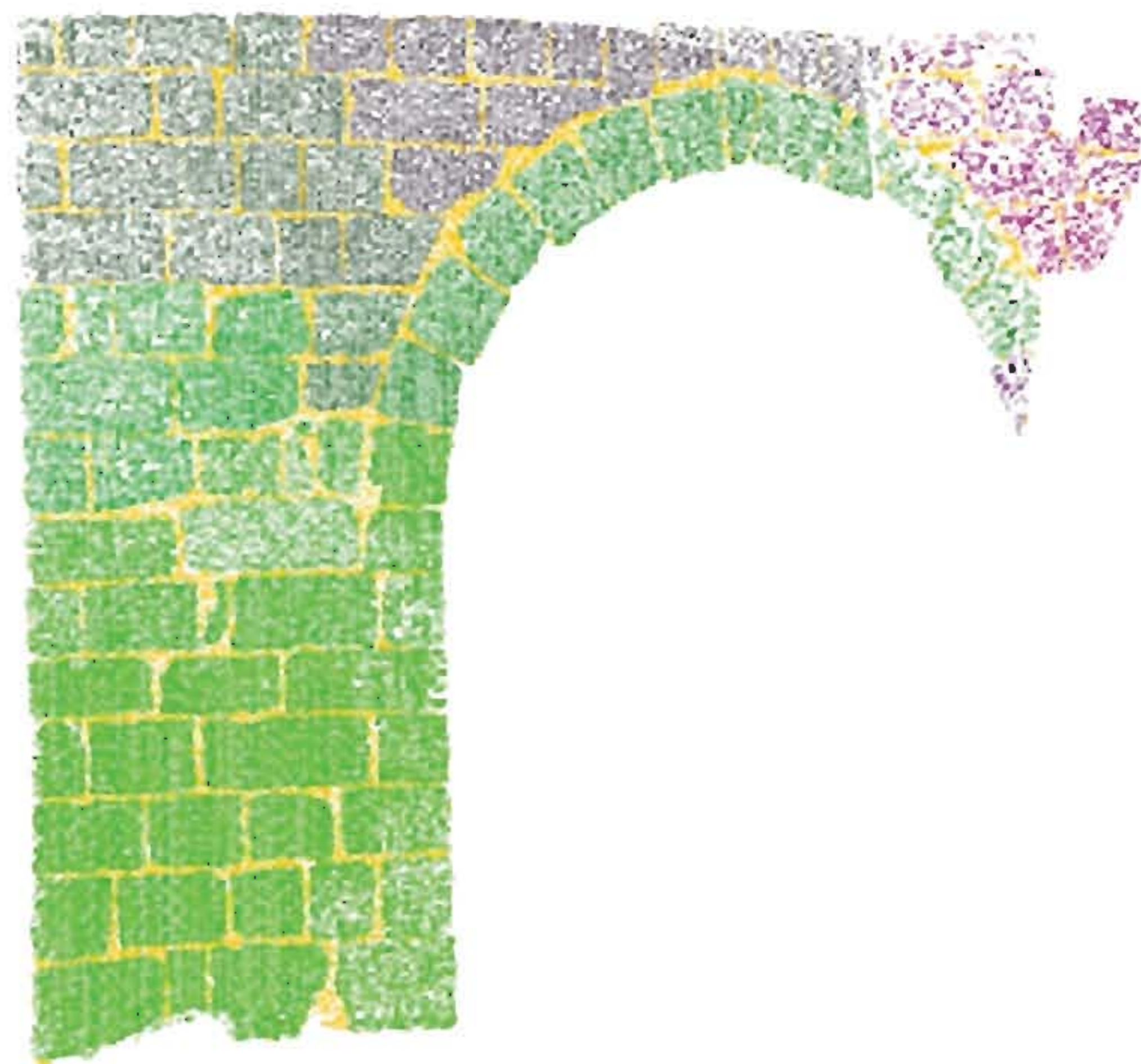
Fig. 19 3D cloud point generation based on autocorrelation where semantic information is used to obtain a colour.
