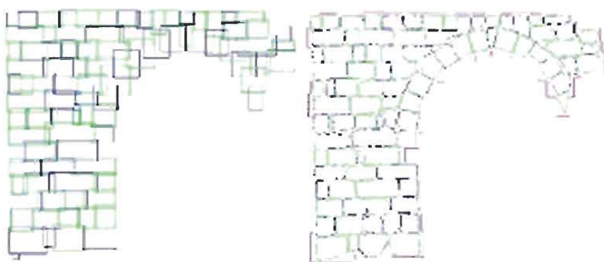
Fig. 7 Blocs bounding boxes scaled at 1.25 (left) and the computed perimeter displayed in magenta (right) superposed with the original blocs.
