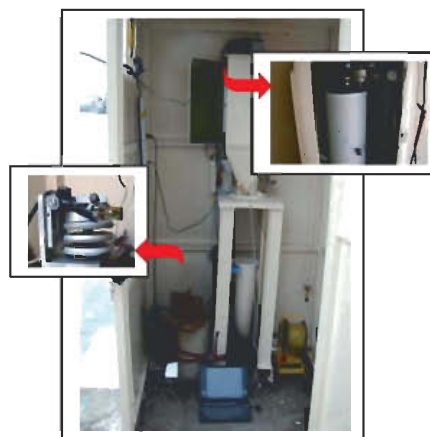
Fig. 1 Tidal gauge site of Algiers sheltering the two tide gauges electronic (in the left) and analogical (in the right).
