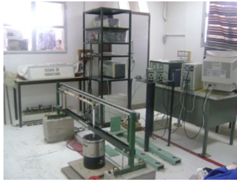
Fig. 1. Set-up Schematic of the modal testing.
