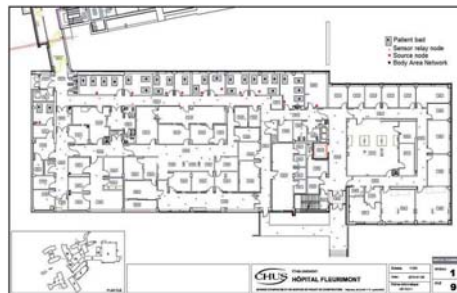
Figure 2: Illustrative diagram of the network architecture in a wing of the Fleurimont CHUS hospital [4].
