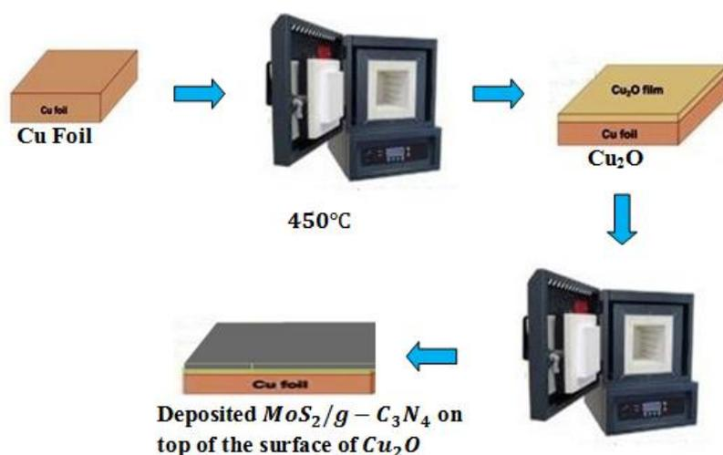
Figure 1. Schematic of a growing  $MoS_2/g - C_3N_4/Cu_2O$  film.
