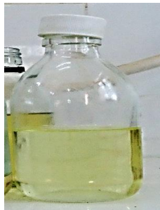
Figure 3. Biodiesel produced from used frying oil.
