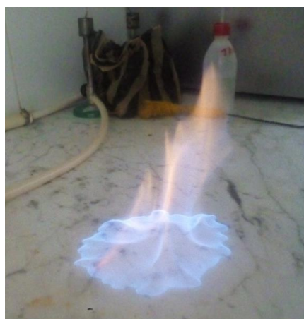
Figure 04: Flame obtained after the combustion of bioethanol
