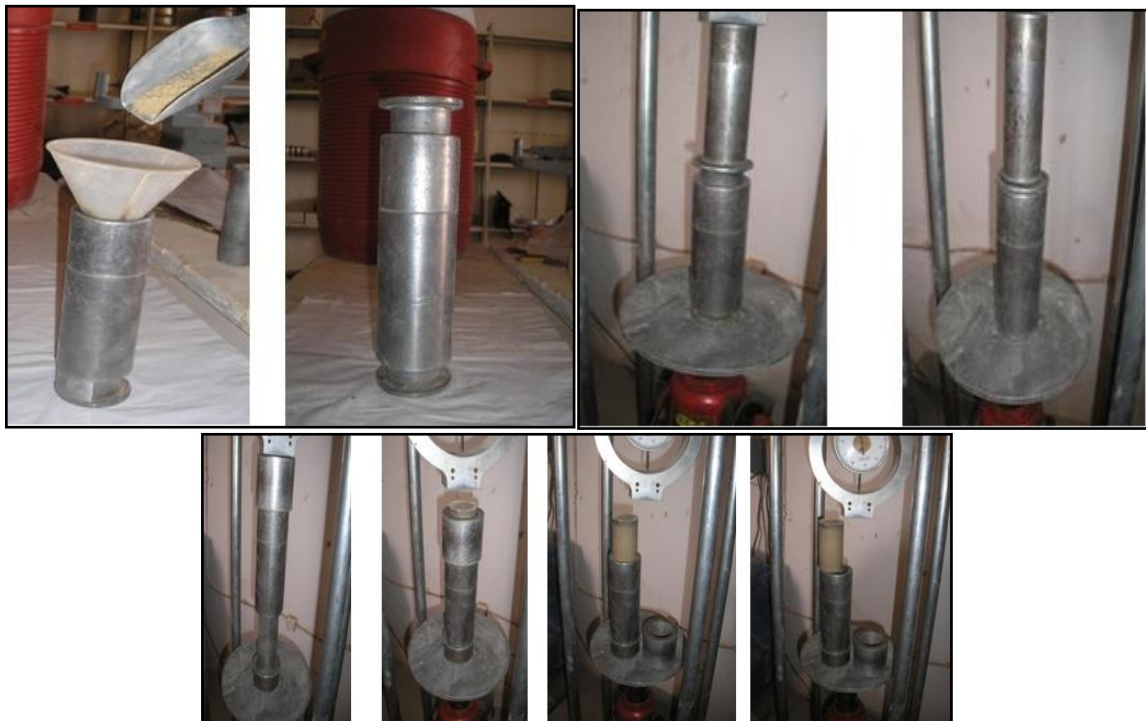
Figure 4. Steps for making cylindrical test pieces for simple compression testing
