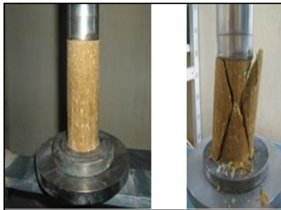
Figure 11. Tuff / sand dune mixture specimen subjected to the compression test.
