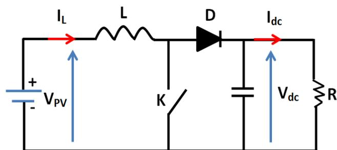
Figure 4. DC-DC Boost converter
