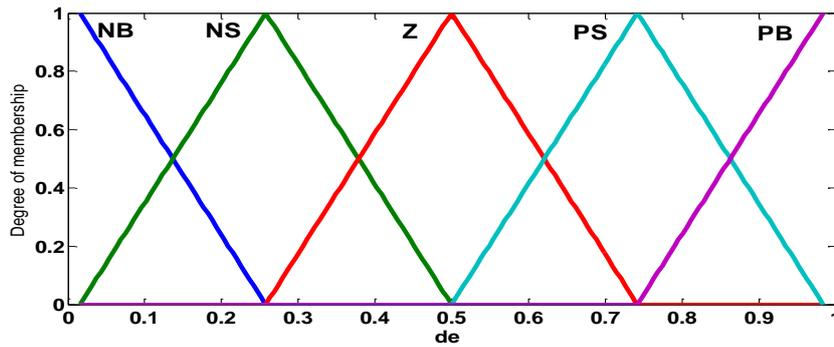
Figure 8. The Membership function of input  $\Delta e(k)$
