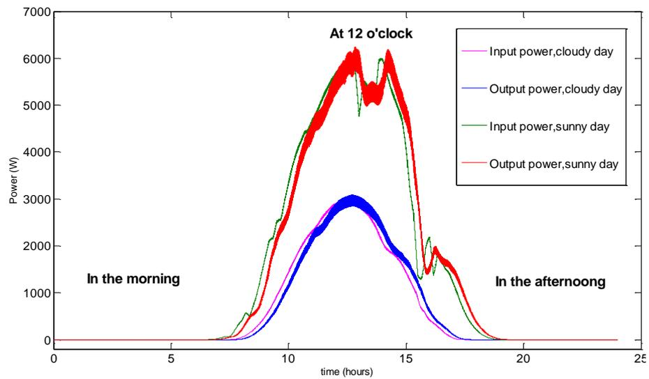
Figure 18. Evolution of input and output power (cloudy and sunny day)
