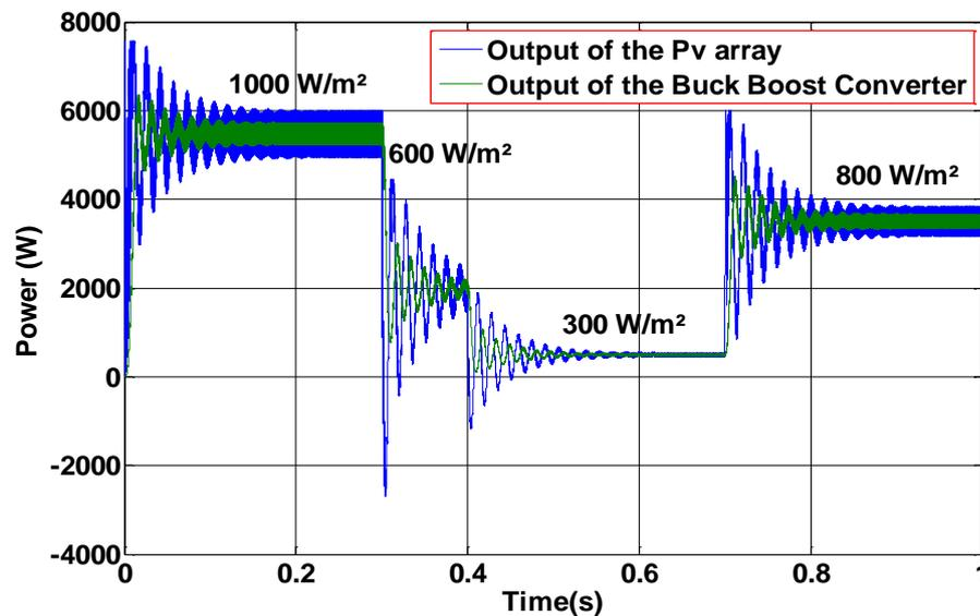
Figure 16. Output power of the PV array and boost converter at constant temperature ( $T=25\text{ C}^\circ$ )
