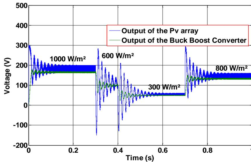
Figure 15. An output voltage of the PV array and boost converter at constant temperature ( $T=25\text{ C}^\circ$ )
