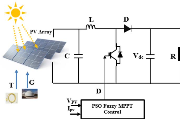
Figure 1. Stand-alone photovoltaic system.
