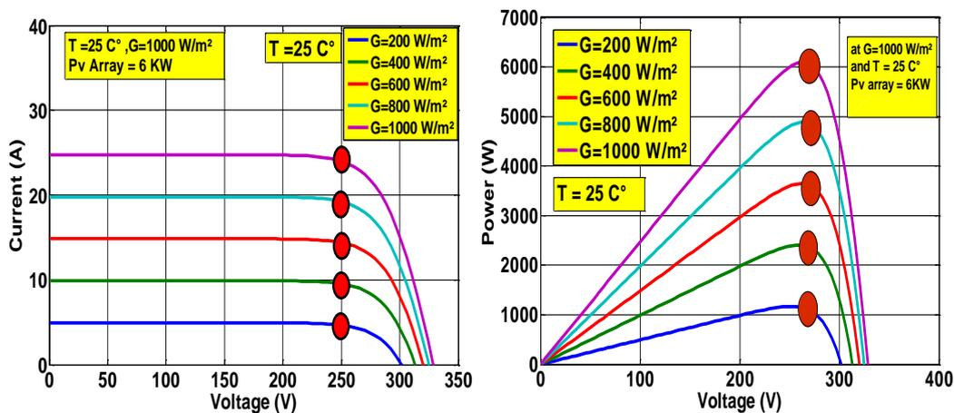
Figure 3. V-I and V-P specific of PV Array (6 kWp) under the change in irradiation
