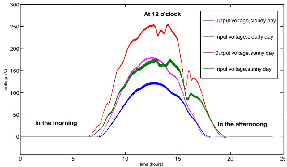
Figure 19. Evolution of input and output voltage (cloudy and sunny day)
