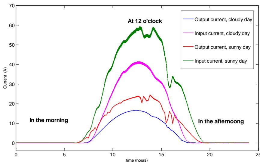
Figure 20. Evolution of input and output current (cloudy and sunny day)
