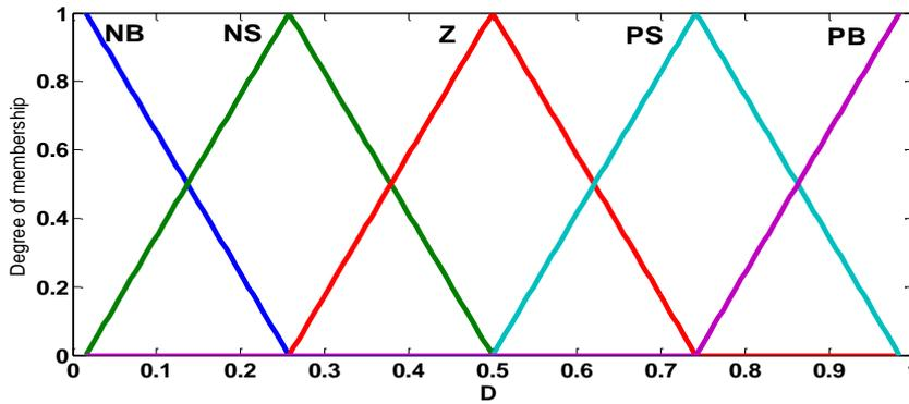
Figure 9. Membership functions of output D (Duty cycle)
