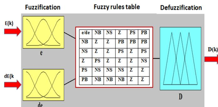
Figure 6. Fuzzy controller configuration
