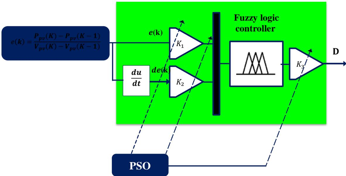
Figure 11. PSO fuzzy MPPT controller Proposed
