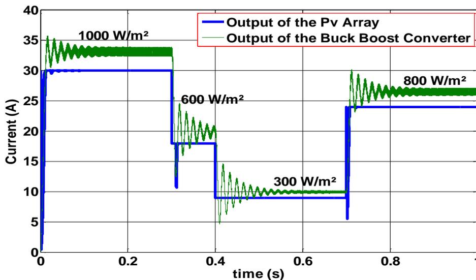
Figure 14. An output current of the PV array and boost converter at constant temperature ( $T=25 \text{ C}^\circ$ )
