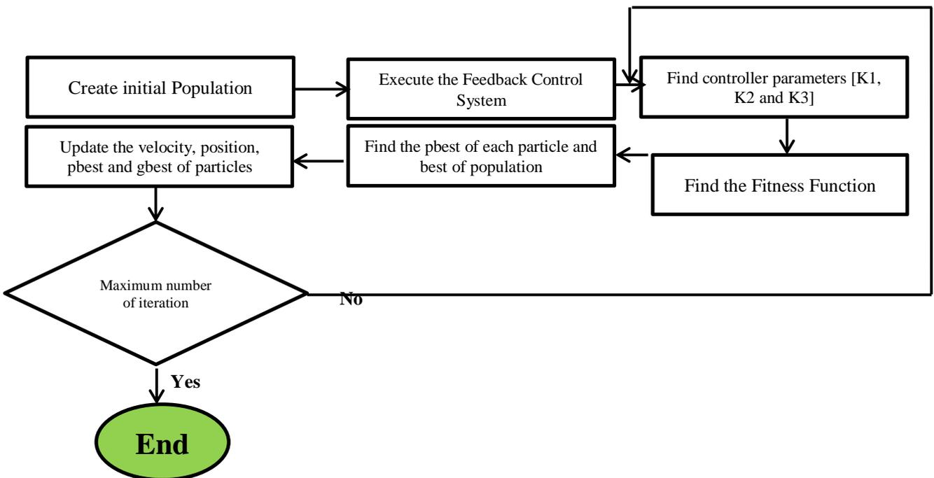
Figure 5. Flow chart of the Proposed PSO Algorithm
