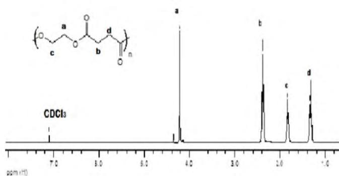
Fig. 2. Nuclear magnetic resonance ( $^1\text{H NMR}$ ) spectra of poly(ethylene succinate).
