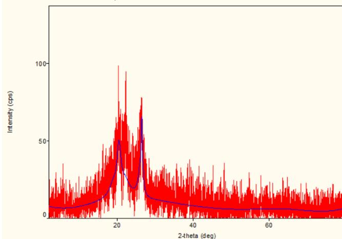
Fig. 3. X-ray diffraction pattern of the PESu.
