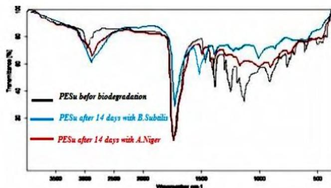
Fig. 5. Infrared spectra of PESu before and after 14 days of biodegradation.
