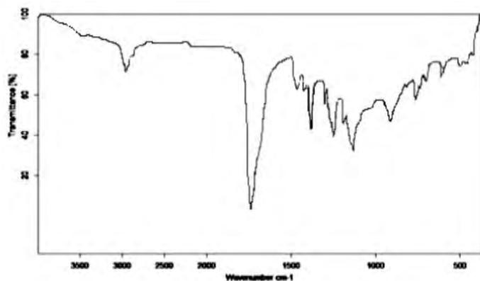
Fig 1. FT-IR spectrum of poly(ethylene succinate).
