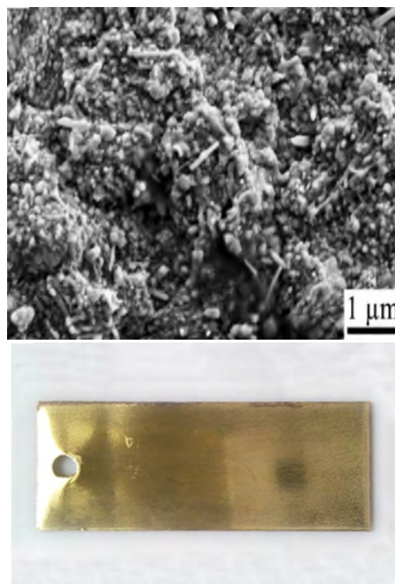
Fig. 4. SEM images of Cu-Zn deposits obtained after heat treatment at 400^\circ\text{C} for 1h and photograph of Cu-Zn film obtained.
