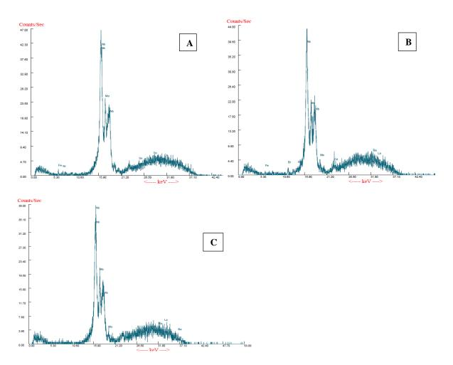
Figure 3: XRF Results Pattern after immersion of mild steel, A= Effluent, B= Seawater and C= Fresh water
