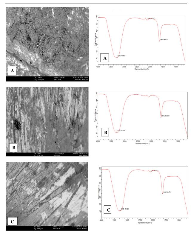
**Figure 1.** SEM Micrograph of mild steels immersed. in different water environments
