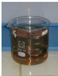
Figure 07: Phenomenon observed in the case of our tests on catechol (Appearance of coloration)
