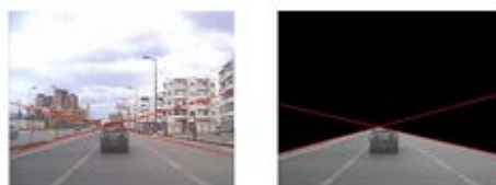
Fig.3. Interval Research obtained after edge detection by the operator "Canny".
