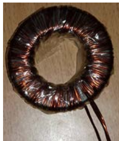
Fig. 9. Realized coil of 2.48 mH.
