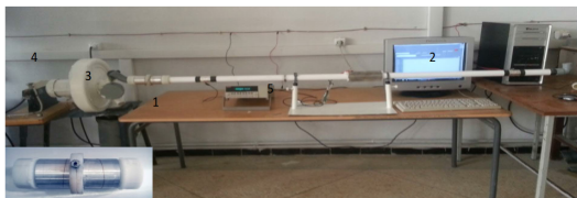
Fig. 3. The experimental setup 1 : faraday cage— 2 : measuring instrument— 3 : Aspiration motor — 4 : speed controller -5: electrometer (model 6415, Keithley Instruments)
