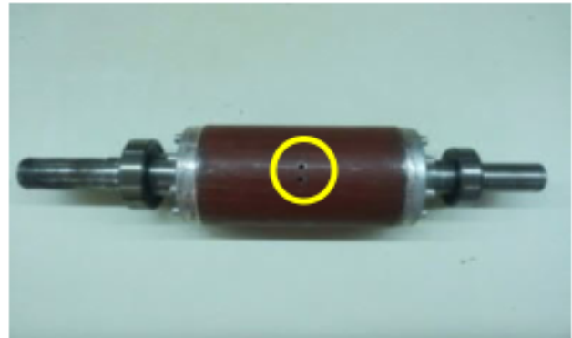
Fig. 3. Squirrel cage rotor with two broken bars.
