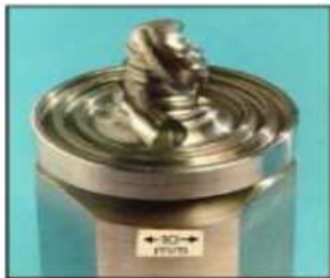
Figure 2 : Outil de soudage FSW [4]
