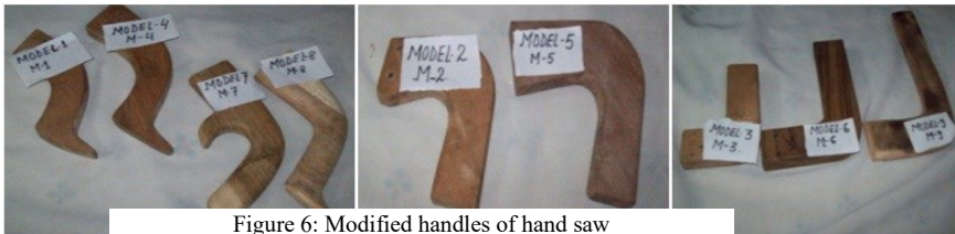
Figure 6: Modified handles of hand saw
