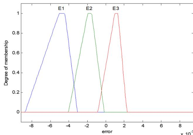
Fig. 7 the membership functions for input 1 (error)
