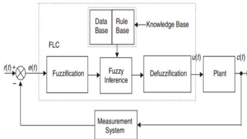
Fig. 1 Block diagram for a fuzzy logic controller
