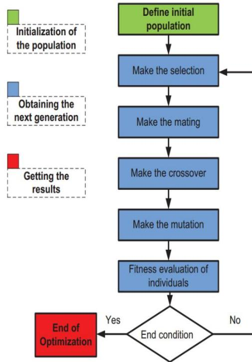
Fig. 3 General mechanism for GA computation
