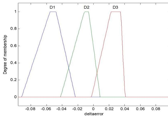
Fig 8 the membership functions for input 2 (Delta error)
