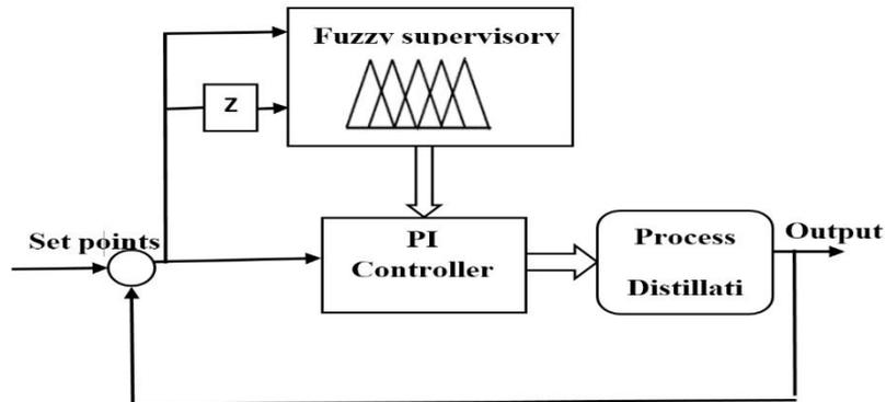
Fig. 2 Block diagram for a PI fuzzy supervisory PI I controller
