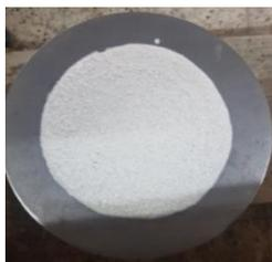
**Figure 2.** Essai de la consistance.
