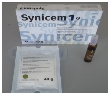
Fig. 2. Two components of PMMA: powder (polymer) and liquid (monomer) are mixed in a ratio of 2 g : 1 ml (Synicem 1G, REF 880223).
