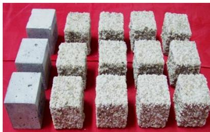
**Figure 4:** Deterioration of specimens after 7 weeks of immersion in: (1) Tap water, (2) molar acid (3.4:1) solution.
