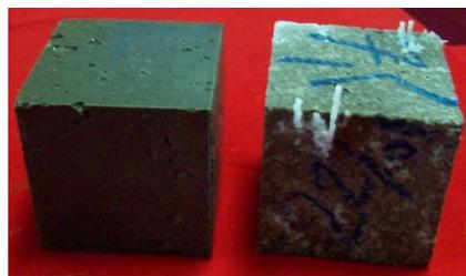
**Figure 3:** Deterioration of specimens after 7 weeks of immersion; (1) Tap water, (2) HF, respectively. (From the left to right).
