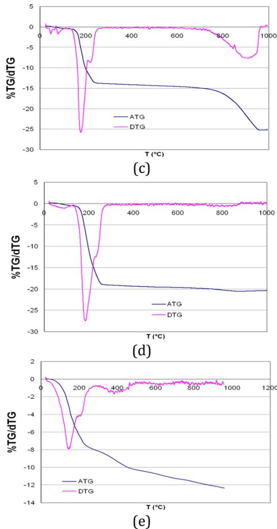
**Figure 5:** TG/dTG curves at 10 K/min of PET0 in: (a) H<sub>2</sub>O, (b) HNO<sub>3</sub>, (c) H<sub>2</sub>SO<sub>4</sub> (d) (3.4:1), (e) HF acids exposure.
