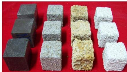
**Figure 2:** Deterioration of specimens after 7 weeks of immersion; (1) Tap water, (2) H<sub>3</sub>PO<sub>4</sub>, (3) HNO<sub>3</sub>, (4) H<sub>2</sub>SO<sub>4</sub>, respectively. (From the left to right).
