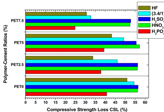
**Figure 1:** CSL (%) of specimens under acid solutions exposure.
