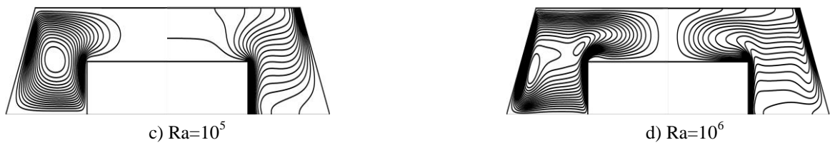
Fig.4. Streamlines and isotherms for annulus Aspect ratio Ar=1 , K=2 , \chi=0.5 and \delta=70^\circ .
