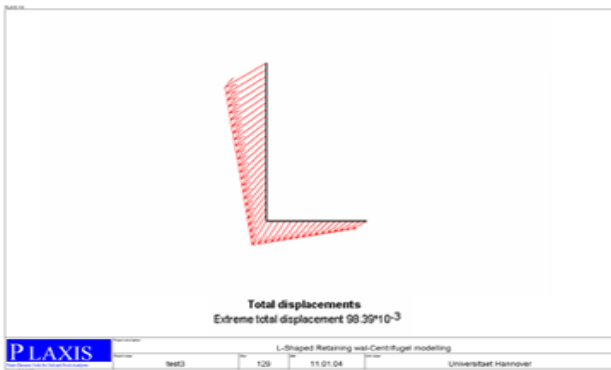
Figure 9: wall total displacement vectors.
