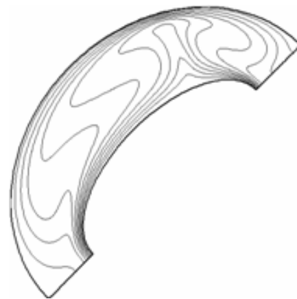
FIG. 8 Isotherms for e_1=0.86 , Fr=5 , \alpha=45^\circ and Gr=5.10^4
