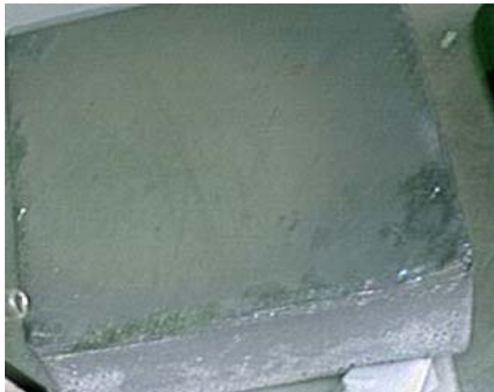
Fig. 3: 44 cm square cross section multi-crystalline silicon ingot
