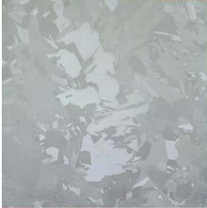
Fig. 5: Grain shape of 10 cm square multi-crystalline silicon wafer
