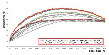
Fig. 4: Variation of measured absorber plate temperatures and water temperatures with local time, for the conventional cooker and improved cooker used without, with one and two booster mirrors.
