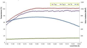
Fig. 3: Variation of measured water temperatures with global solar radiation for both solar cookers (17/02/2013) used to determine the second figure of merit
