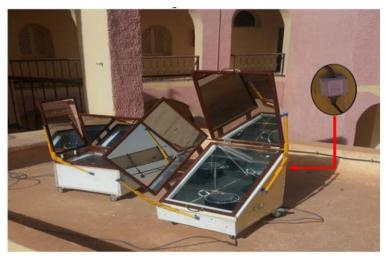
Fig. 1: View of realized box type solar cookers
