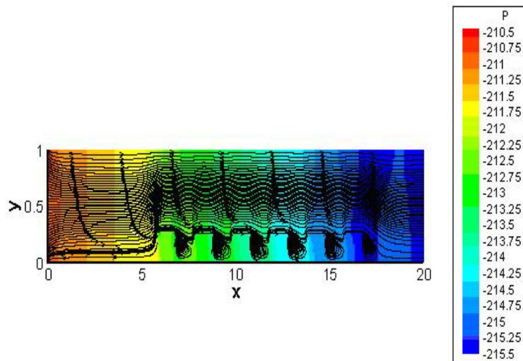
Fig. 2: Pressure field and streamlines of the air cooling when the channel is not filled with a porous medium. We notice the presence of clockwise rotating vortices between the blocks.
