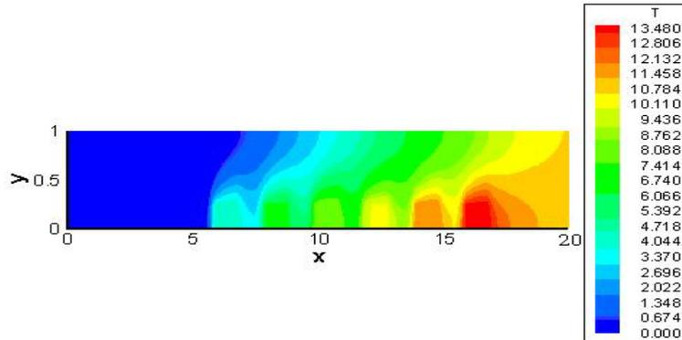
Fig. 5: The thermal field of the air cooling in the channel filled with a porous medium with  $Da = 10^{-9}$ . We notice the reduction of the temperature level and the increase of the transversal thermal mixing compared to those of the reference state.
