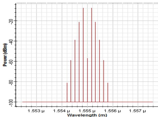
Figure 12. Signal spectrum of the signal at the output of the Mach-Zehnder modulator in the first block.
