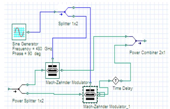
Figure 5. The second OTDM multiplexer
