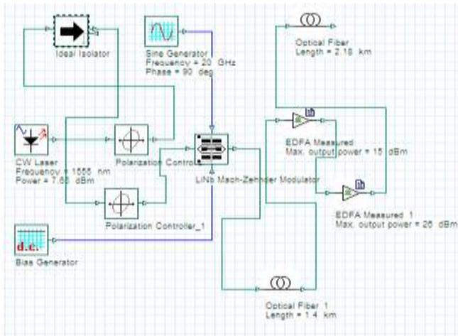
Figure 2. Optical source of breves pulse at 40 GHz
