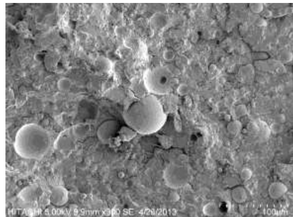
Figure 7. From first to last graph: (1) SEM image of 20% FA-UP tensile test specimen, (2) 40% FA-UP impact specimen, and (3) Fig. 2: SEM-EDX analysis of a chosen particle..
