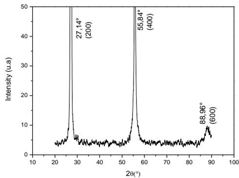
Fig. 1 XRD pattern of pure KCl single crystal
