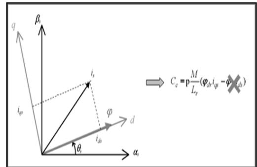
Figure.4 Principle of Vector Control.
