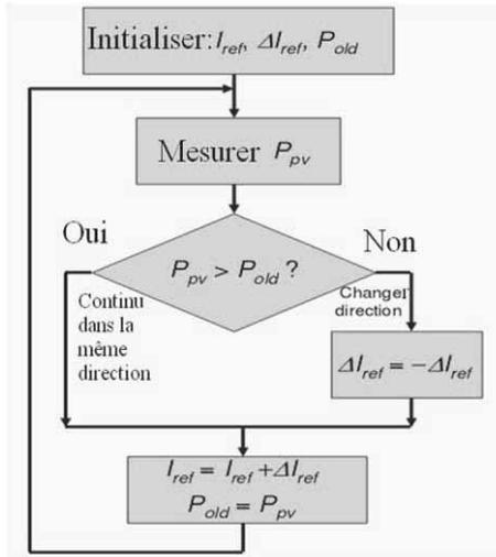
Figure.2 The P&O MPPT algorithm.
