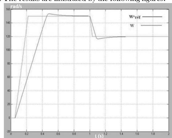
Figure.7 Rotor speed "ω" and its reference.
