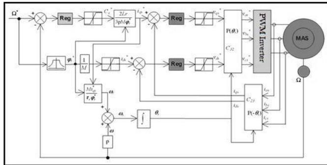
Figure.5 Speed control of induction motor in FOC.
