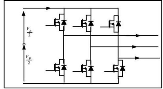
Figure.3 Voltage PWM Inverter.
