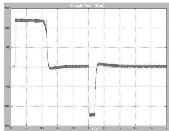
Figure.8 The electromagnetic torque and its reference.
