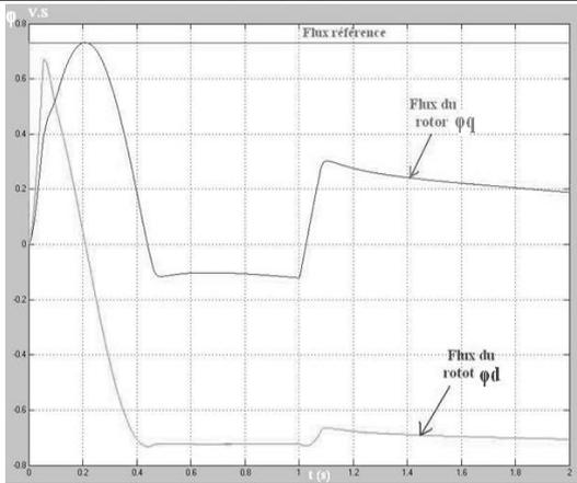
Figure.9 The quadratic and direct rotor flux.
