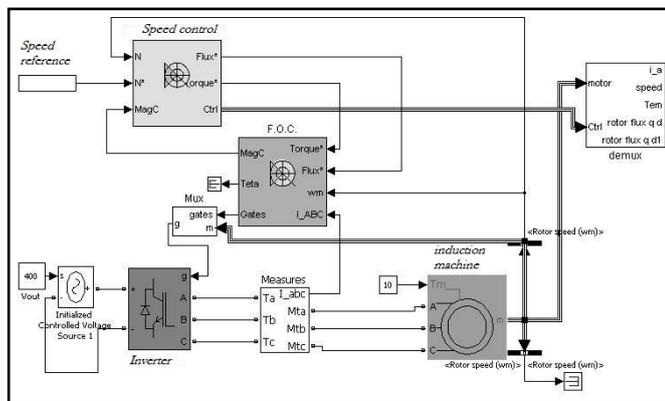
Figure.6 Bloc of flux oriented control in SIMULINK
