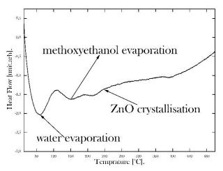
Figure 4. DSC thermogram of ZnO.
