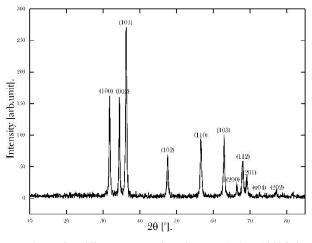
Figure 2. Diffractogram of ZnO annealed at 400°C for 2h.
