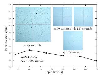
Figure 5. Evolution of film thickness according to spin time. a), b), c) and d) are images taken by optical microscope at 5X magnifying of a 2mm area.
