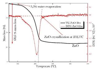
Figure 3. TG and DTG thermograms of ZnO.
