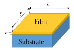
Figure 1. Schematic of ZnO thin-film deposited on glass substrate.
