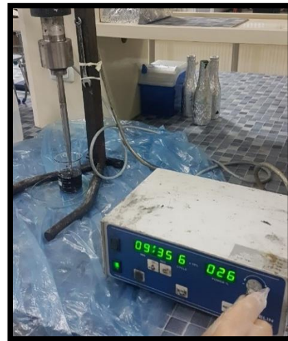
Figure 1. Dispersion of MWCNT within PMMA solution by an ultrasonic homogenizer
