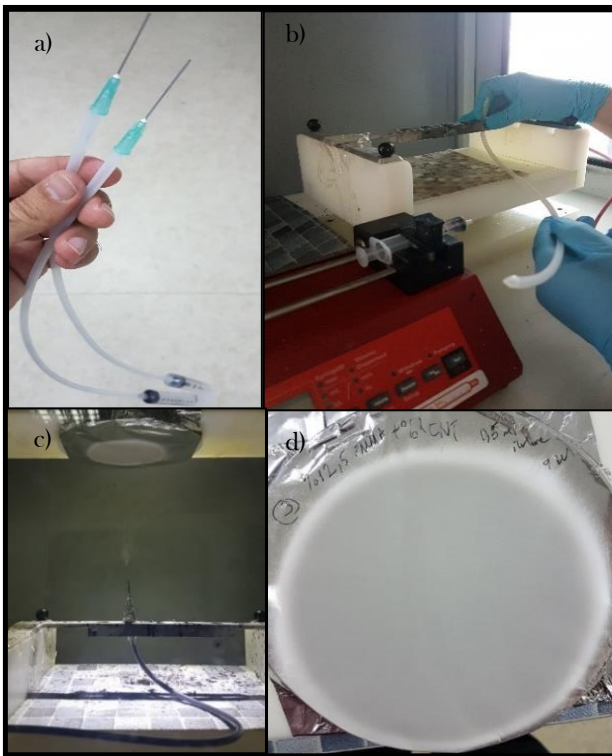
Figure 2. Electrospinning process of PMMA/MWCNT solution a) preparation of injectors, b) system set-up, c) electrospinning of solution and d) 12.5 % wt. PMMA+1% wt. MWCNT nanofibers
