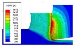
Figure 1. Simulated temperature fields by using the FE model with Lagrangian boundaries [28].
