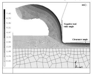
Figure 4. Equivalent plastic strain plot in reference conditions [57].
