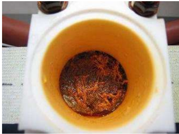
Figure 11. GFRP specimen after corrosion test with bromine.
