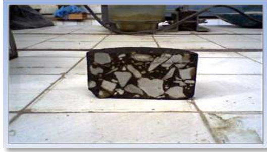
Figure 7. Specimens after storage 48 h in the oven.(Filler 10%)
