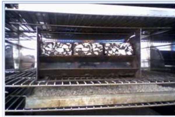
Figure 6. Preserved test-tubes 48h in the drying oven
