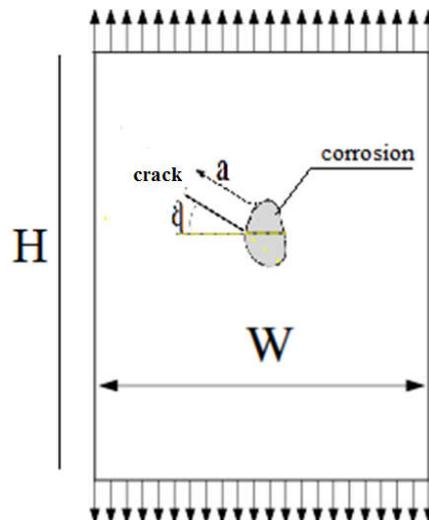
Fig. 1 Geometric model of the corroded cracked plate, repaired by rectangular patch
