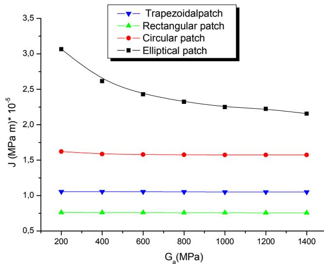
Fig.7. Variation of the J integral as a function of the adhesive shear modulus ( $a = 30\text{mm}$ ,  $\theta = 30^\circ$ )
