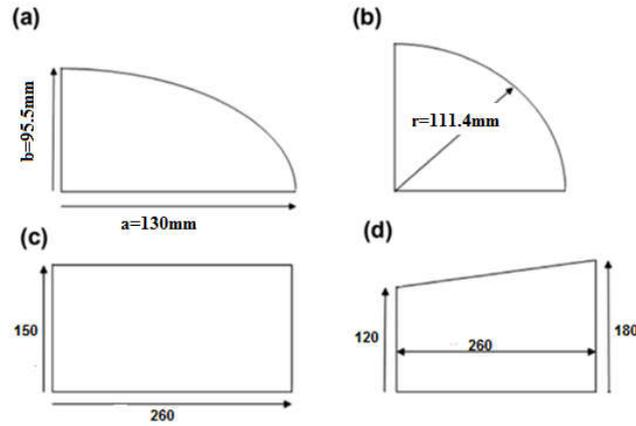
**Fig. 2** Dimensions of the patches (a) elliptical, (b) circular, (c) rectangular and (d) trapezoidal
