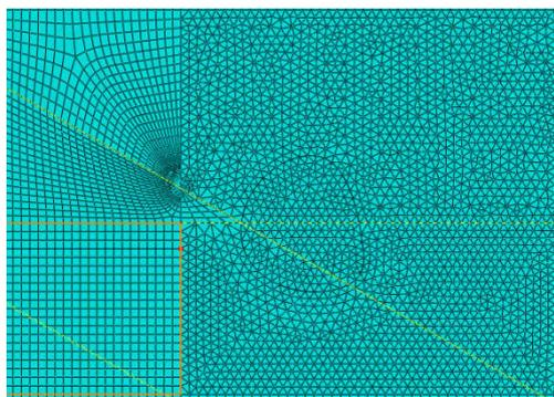
**Fig. 3** Mesh of the plate near the corrosion and inclined crack
