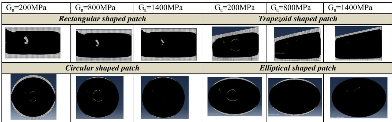
Fig. 4 Damaged area for different of the patch shapes and for different adhesive shear modulus (a)  $G_a = 200\text{MPa}$ , (b)  $G_a = 800\text{MPa}$  and (c)  $G_a = 1400\text{MPa}$
