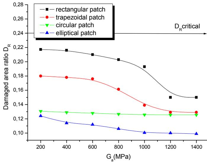
Fig.6 Ratio of damaged area vs the adhesive shear modulus for different patch shapes.
