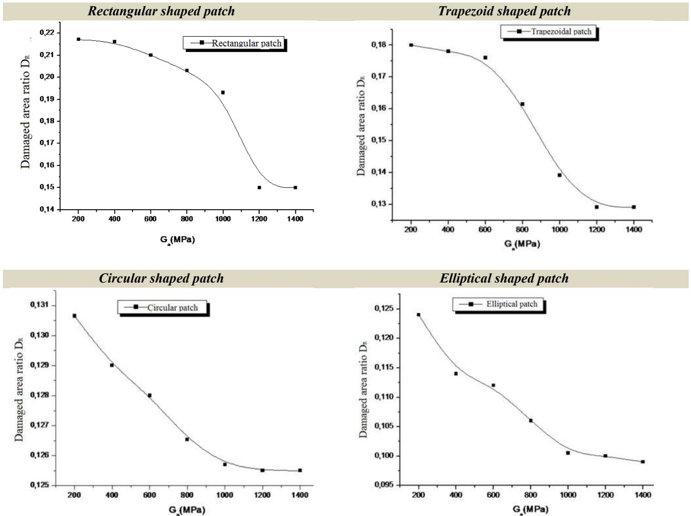
Fig. 5 Variation of the damaged area ratio versus the adhesive shears modulus.
