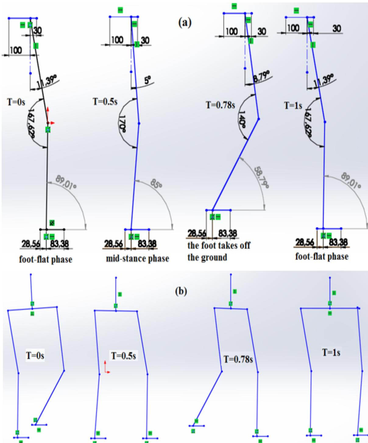
Fig. 5-Simulation of one gait cycle of bipedal robot by using SolidWorks2015 (a) the right leg, (b) the two legs
