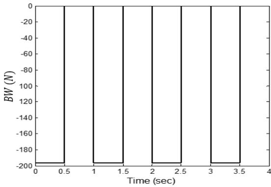
Fig. 6-The (BW) applied at the right ankle in (-z) direction during walking
