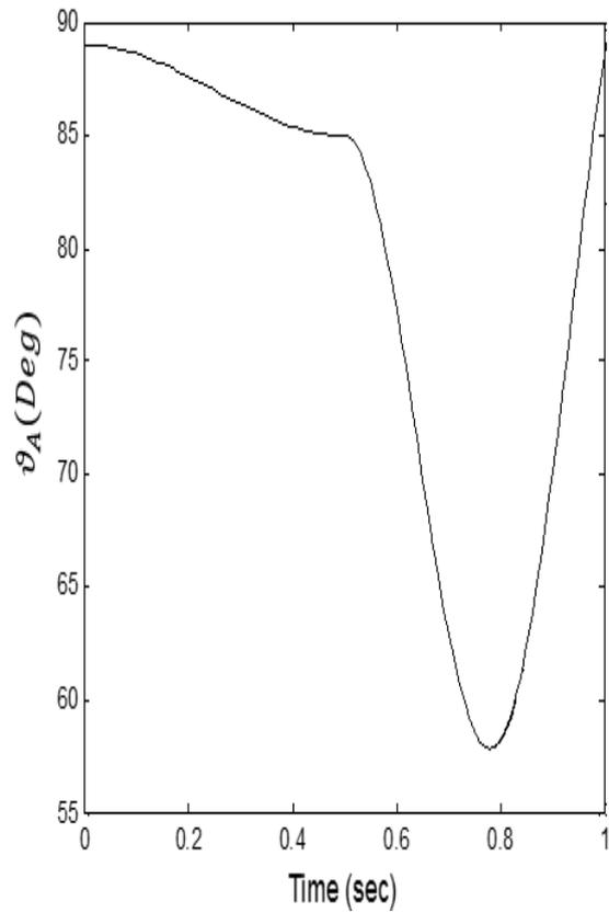
Fig. 4 -Motion pattern of the ankle joint
