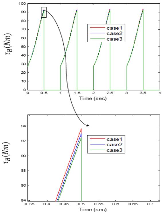
Fig. 8-The torque patterns at the hip joint
