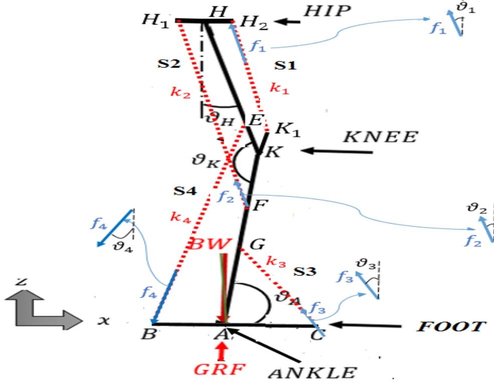
Fig.1-Bipedal locomotion model with compliant legs (only one of the two legs is shown in this figure)
