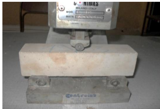
Fig 1. Three point bending test equipment
