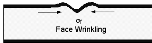
Fig 3. Face wrinkling failure mode
