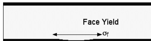
Fig 2. Face yielding failure mode
