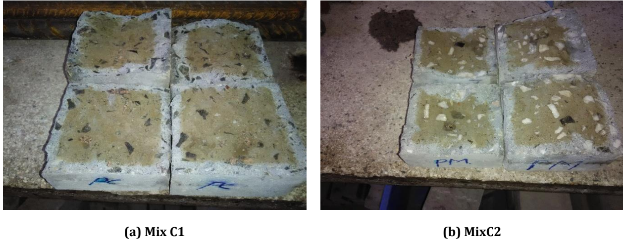
Fig 2. Images of chloride ion penetration of concrete.
