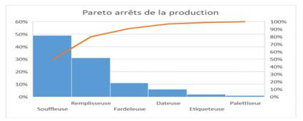
According to the analysis, the blower and filler are the two manufacturing line stoppages. This finding emphasizes the need of prioritizing maintenance and upgrade efforts on these two critical pieces of equipment. By
