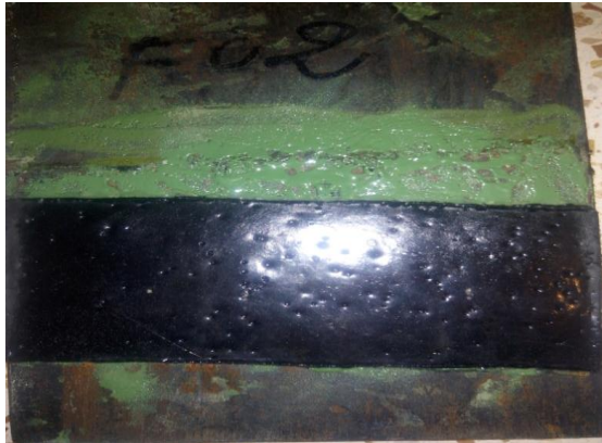
Figure 1. Three-layer coating on a metal substrate
