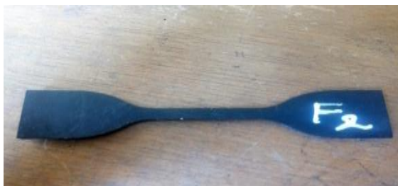
Figure 2. Tensile test sample of a HDPE-porcelain mixture after shaping in the injection molding machine
